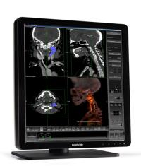
Nio Color 3MP LED is a 3 MegaPixel high-bright color display system with LED backlights, providing excellent image quality for confident diagnoses. Nio Color 3MP LED provides an effective display solution for a multitude of applications and modalities, including 3D PACS, 3D echo, ultrasound, orthopedic imaging, CAD, image fusion, nuclear medicine and PET.
