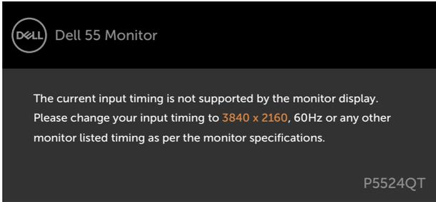
This means that the display cannot synchronize with the signal that it is receiving from the computer. See [Display Specifications](#) for the Horizontal and Vertical frequency ranges addressable by this display. Recommended mode is 3840 x 2160.
