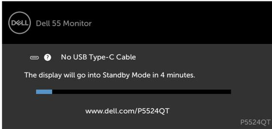
4. This box also appears during normal system operation, if the video cable becomes disconnected or damaged.
