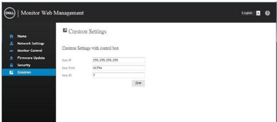
Configures the setting of **Crestron** control system devices.
