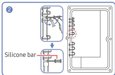
Remove the appropriate silicone bar for the thickness of the cable to connect.
