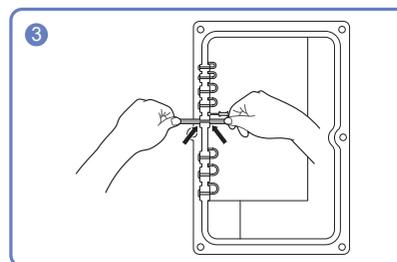
Insert the appropriate cable into the hole from which the silicone bar was removed.
