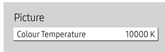
It sets colour temperature. The value and temperature increase simultaneously, so the ratio of blue colour rises. (Range: 2800K-16000K)
