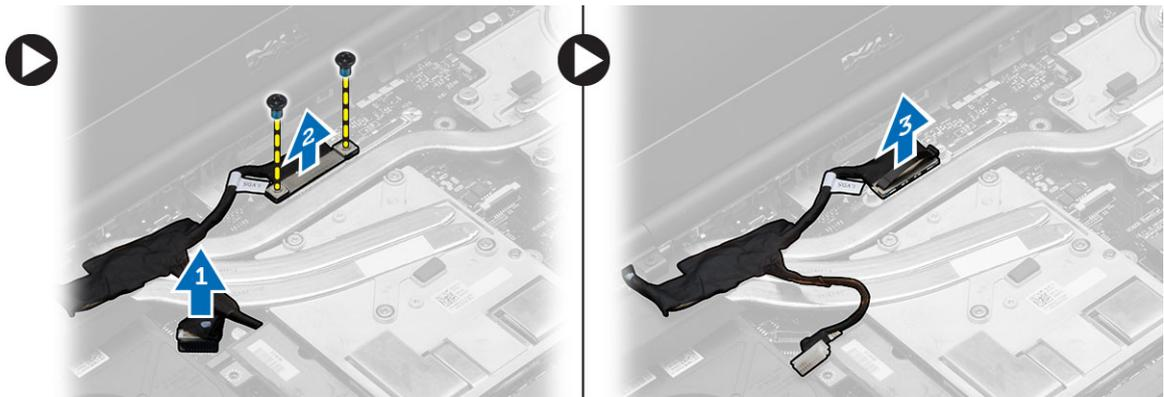
7. Remove the screws that secure the display assembly to the computer. Remove the display assembly from the computer.
