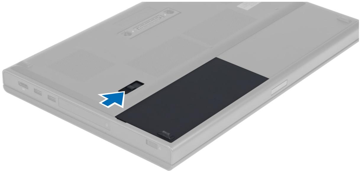
3. Lift and remove the battery from the computer.
