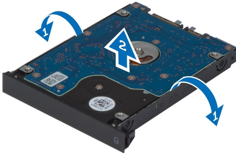
**NOTE:** A rubber filler is installed to the hard-drive bracket for 7 mm hard drives. It is designed to prevent vibrations and for correct installation of the 7 mm hard drives. 9 mm hard drives do not require the filler when installed into the hard-drive bracket.
