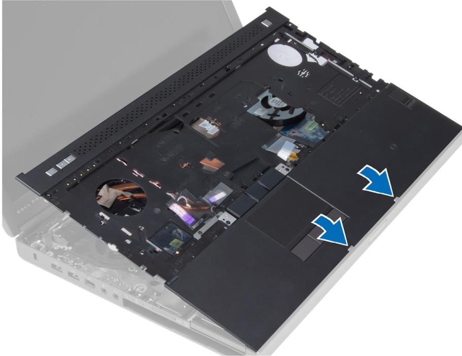
2. Tighten the screws that secures the palmrest to the computer.
