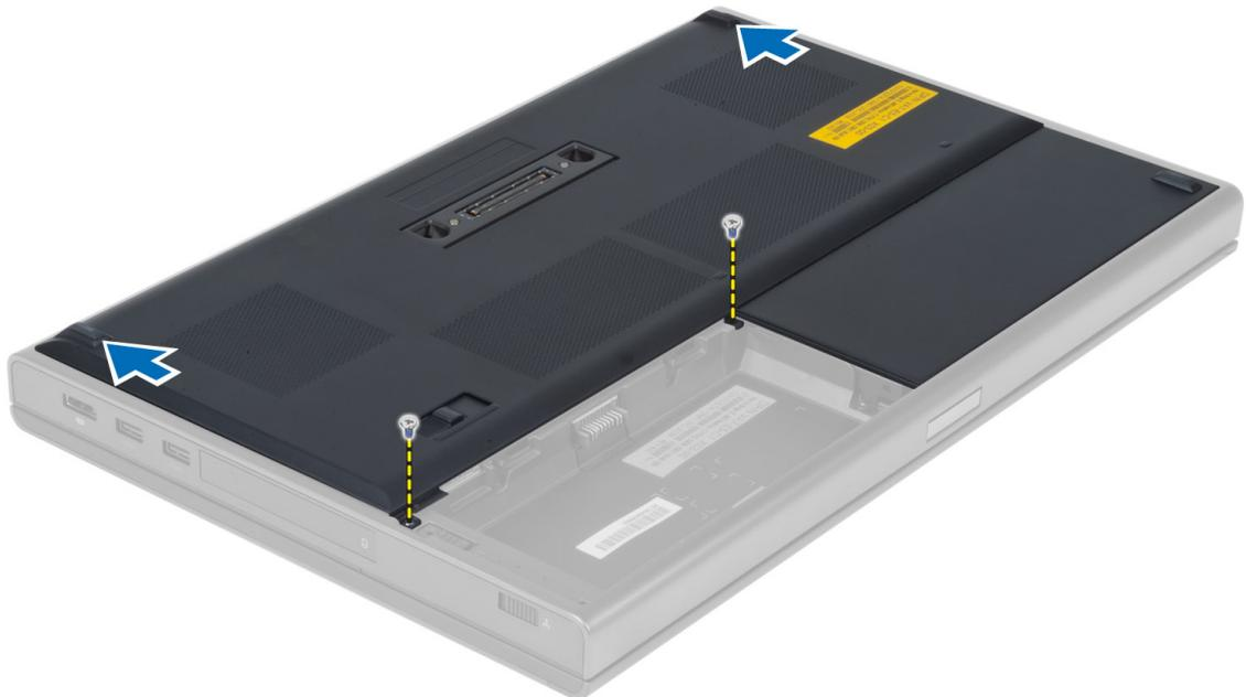
4. Lift and remove the base cover from the computer.
