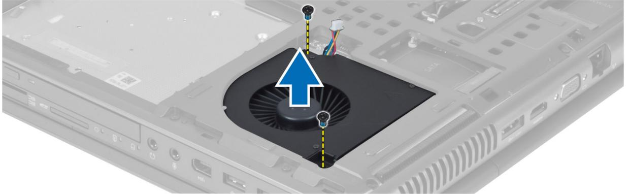
4. Disconnect the processor-fan cable.
