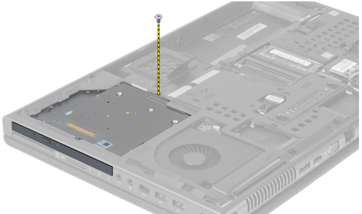
4. Pry and slide out the optical drive to remove it from the computer.
