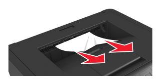
2 From the printer control panel, select Next > OK > Clear the jam, press OK > OK to clear the message and continue printing.
