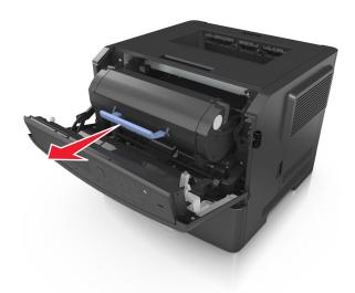
**3** Lift the blue handle, and then pull the imaging unit out of the printer.
