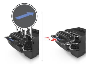
**8** Insert the toner cartridge by aligning the side rails of the cartridge with the arrows on the side rails inside the printer, and then insert the cartridge into the printer.
