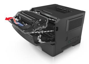
**Warning—Potential Damage:** Do not touch the shiny blue photoconductor drum under the imaging unit. Doing so may affect the quality of future print jobs.
