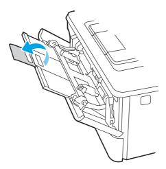
4. Press down on the tab on the right paper guide, and then spread the paper guides to the correct size.
