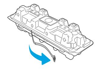
5. Remove the toner cartridge from the opened packaging shell. Place the used toner cartridge in the shell for recycling.
