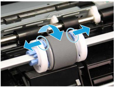
Figure 6-12 Release the roller
