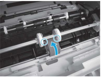
Figure 6-15 Install the roller
