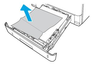
**3.** Verify that the rear paper guide is adjusted to the indentation for the correct paper size. If necessary, pinch the release and move the rear paper guide to the correct position. It should click into place.
