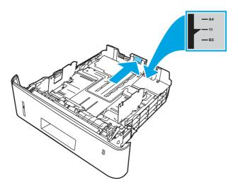
**9.** Load the paper into the tray. Make sure that the stack is flat at all four corners and that the top of the stack is below the maximum-height indicators.
