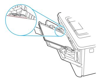
6. Press down on the tab on the right paper guide, and then adjust the paper guides so that they lightly touch the paper stack but do not bend the paper.
