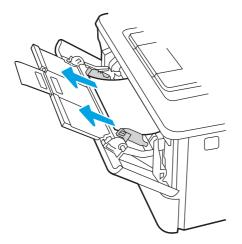
2. Adjust the paper guides to the correct paper size, then .reload paper into the tray.
