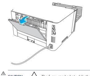
**CAUTION:** The fuser can be hot while the printer is in use. Wait for the fuser to cool before handling it.
