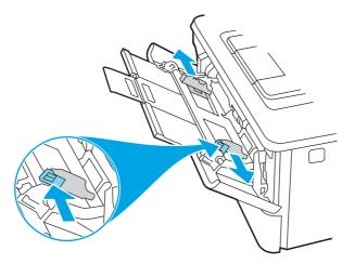
5. Load the paper into the tray. Make sure that the paper fits under the tabs and below the maximum height indicators.
