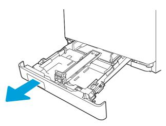
2. Adjust the paper-width guides by squeezing the adjustment latches on the guides and then sliding the guides to the size of the paper being used.
