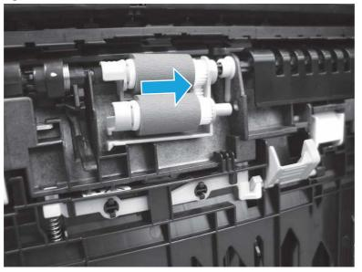
Figure 6-22 Install the roller holder
