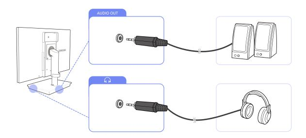
Connect an audio output device (headphones or speakers) to [AUDIO OUT] on the back or  $[\,\widehat{\mathbf{h}}\,]$  on the right side of the stand base.
