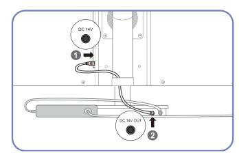
Connect the power extension cable to [DC 14V] on the monitor and [DC 14V OUT] on the stand base.
