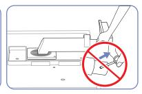
Do not remove the fixing pin until you are finished attaching the stand.
