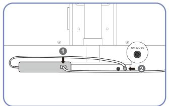
Connect the power cable to the DC power adapter. Next, connect the DC power adapter to [DC 14V IN] on the stand base.
