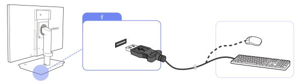
1 Connect a USB device (keyboard, mouse, etc.) to  $[\ref{V}]$  on the back or right side of the stand base.
