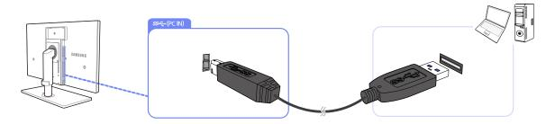
Connect the USB cable to [ ] on the back of the product and USB [ ] on the PC.
