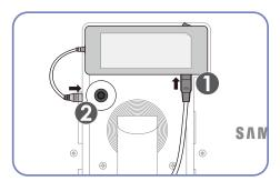
Connect the power cable to the DC power adapter. Next, connect the DC power adapter to the product.
