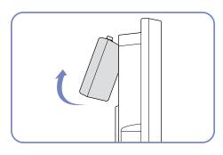
To remove the DC power adapter, lift it outwards from the bottom as shown in the image.
