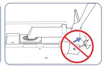
Do not remove the fixing pin until you are finished attaching the stand.
