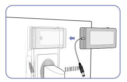
Put the DC power adapter in the groove, with the switch facing upward.
