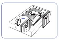
Insert the stand base into the stand in the direction of the arrow.
