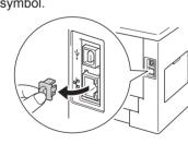
**b.** Connect the network interface cable to the Ethernet port and then connect it to a free port on your hub.
