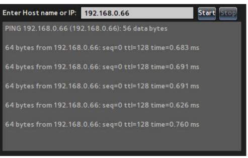
Using the Ping command, you can check the status of the network connection for the IPs entered.
