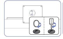
Fasten the screw tightly (using a screwdriver or coin) into the bottom of the stand base.
