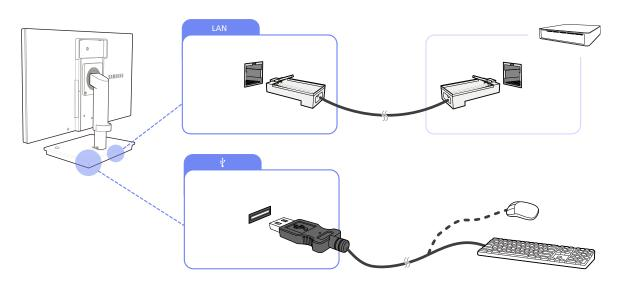
1 Connect the [LAN] port on the back of the stand base to the server using the LAN cable.
