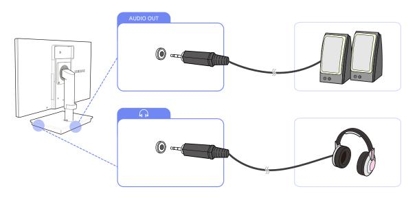
1 Connect an audio output device (headphones, speakers, etc.) to the [AUDIO OUT] port on the back or the [ $\bigcap$ ] port on the side of the stand base.
