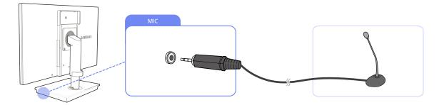
1 Connect the microphone to [MIC] on the right side of the stand base.
