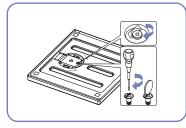
Fasten the screw tightly (using a screwdriver or coin) into the bottom of the stand base.
