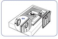
Insert the stand base into the stand in the direction of the arrow.
