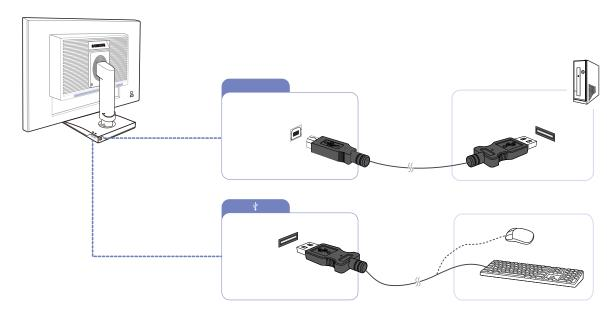
1 Connect the **o** port of the monitor and the USB port of the computer with the USB cable.
