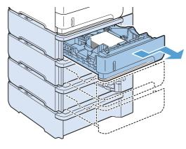
2. If the edge of the jammed paper is visible in the feed area, slowly pull the paper down and out of the product. (Do not pull the paper straight out, or it will tear.) If the paper is not visible, look in the next tray or in the top-cover area.
