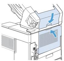
4. If a jam message persists, a sheet is still jammed. Look for it in another location. Check the front of the accessory and carefully remove any jammed paper.
