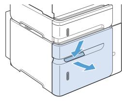
2. If paper is in the tray, remove it. When paper is in the tray, the guides cannot be adjusted.
