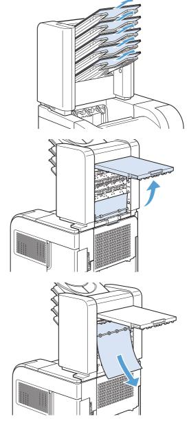
4. If the paper is jammed at the bottom of the 5bin mailbox, open the rear output bin, and then pull straight up on the paper to remove it.
