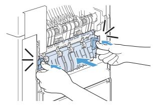
Reinstall the rear output bin. Insert the right hinge-pin into the hole inside the product. Push inward on the left hinge, and slide it into the hole inside the product. Close the rear output bin
