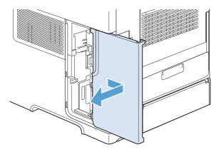
5. Open the access door by pulling on the metal tab.
