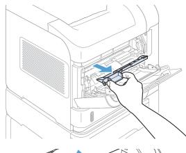
5. Rotate the paper guide to check for additional jammed paper underneath. If jammed paper is present, remove it.
