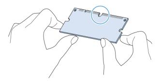
8. Press the DIMM straight into the slot, and press firmly. Make sure the locks on each side of the DIMM snap into place.
