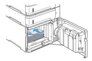
5. Make sure that the height of the stack does not exceed the maximum-height indicators on the guides and that the front edge of the stack is aligned with the arrows.
