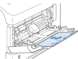
3. Load the paper into the tray. Make sure that the paper fits under the tabs and below the maximum-height indicators.
