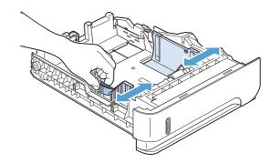
3. Pinch the release lever that is located on the rear paper guide and slide it to the correct paper size.
