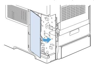
10. Reinstall the right-side panel. Align the tabs on the panel with the slots in the product, and push the panel toward the front of the product until it latches into place.
