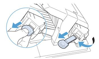
Rotate the green cover on the end of the staple cartridge upward, and remove the jammed staple.
