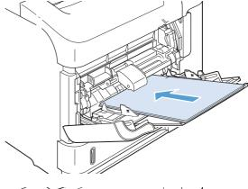
**4.** Adjust the side guides so that they lightly touch the paper stack but do not bend the paper.
