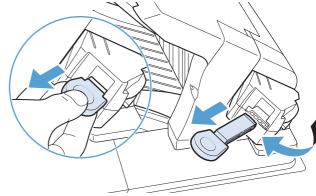
2. Insert the new staple cartridge into the stapler unit and rotate the stapler unit toward the rear of the product until the unit snaps into place.
