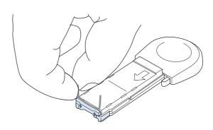
Insert the staple cartridge into the stapler unit, and rotate the stapler unit toward the rear of the product until the unit snaps into place.
