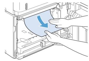
Make sure that the paper does not exceed the fill marks on the paper guides, and that the front edge of the stack is aligned with the arrows.
