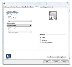
In the Booklet layout drop-down list, click the Left binding or Right binding option. The Pages per sheet option automatically changes to 2 pages per sheet.
