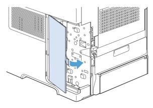
7. Reinstall the right-side panel. Align the tabs on the panel with the slots in the product, and push the panel toward the front of the product until it latches into place.
