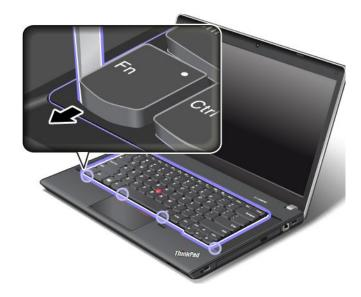
7. Turn the computer over and lock the keyboard frame.
