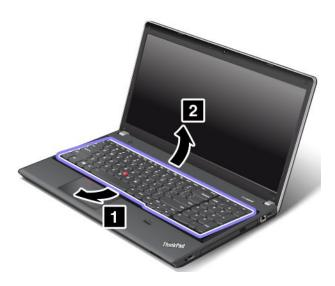
9. Gently put the keyboard on the palm rest and detach the connectors. Then remove the keyboard.
