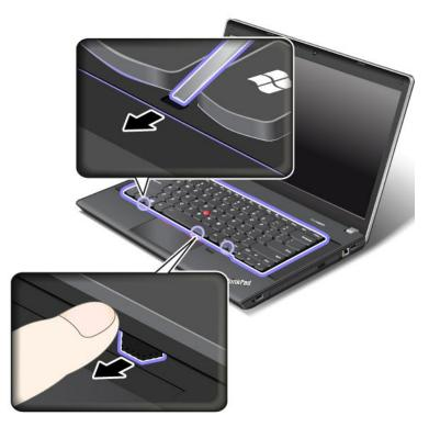
6. Adjust the keyboard frame in place with the keyboard multi-tool and ensure that all the latches are secured under the keyboard bezel.
