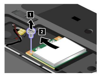
7. Align the contact edge of the new card with the corresponding socket 1. Pivot the card until you can snap it into place. Secure the card with the screw 2.
