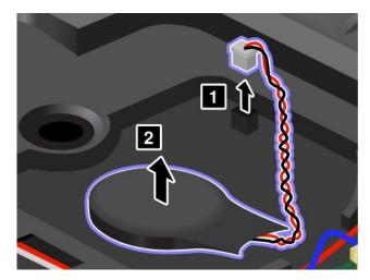
6. Install the backup battery 1. Then attach the connector 2.
