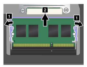
6. Place the notched end of the new memory module toward the contact edge side of the memory slot, and insert the memory module 1 into the slot at an angle of about 20 degrees. Pivot the memory module downward until it snaps into place 2. Ensure that the memory module is firmly installed in the slot and cannot be moved easily.
