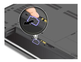
6. To reveal the screw heads beneath the keyboard frame, slide the keyboard frame forward by 2.5 mm (0.1 inch) with the keyboard multi-tool.
