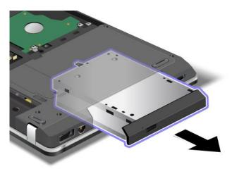
To install a repaired optical drive or a new one, do the following:
