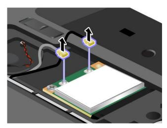
6. Remove the screw 1. The card pops up. Remove the card 2.
