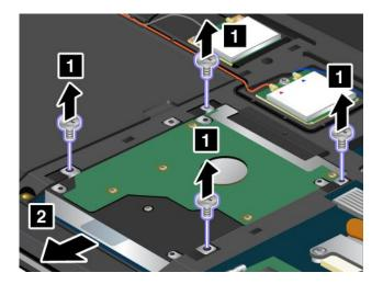
6. Lift the tab to remove the hard disk drive or solid-state drive out of the computer.
