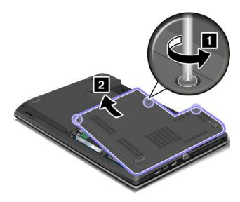
5. Remove the screws 1, and then slide out the hard disk drive or solid-state drive 2.
