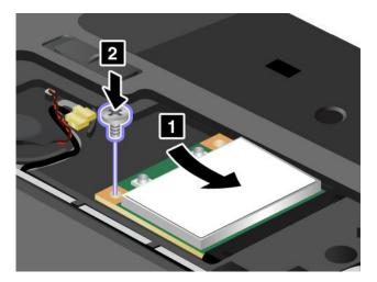
8. Connect the antenna cables to the new card as shown in the drawing.
