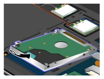
8. Slide the hard disk drive or solid-state drive firmly into the connector 1, and then reinstall the screws 2.
