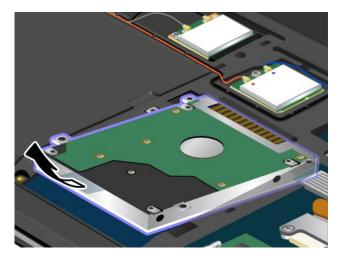
7. Place the new hard disk drive or solid-state drive into the drive bay.
