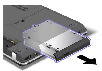
To install a repaired optical drive or a new one, do the following:
