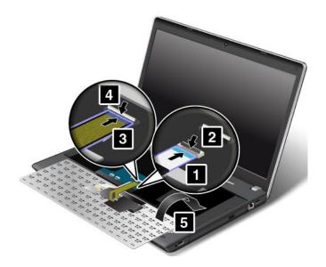
2. Insert the keyboard into the space under the frame of the keyboard bezel as shown.
