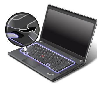
7. Loosen the screws that secure the keyboard with the keyboard multi-tool.
