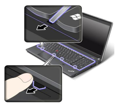
6. Adjust the keyboard frame in place with the keyboard multi-tool and ensure that all the latches are secured under the keyboard bezel.
