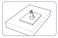
Check if the Stand Connector is firmly connected.
