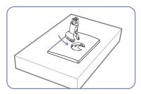
Insert the Stand Connector into the Stand in the direction shown by the figure.
