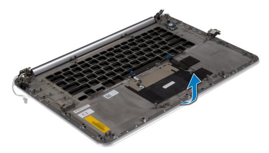
5. Remove the palmrest assembly away from the display assembly.
