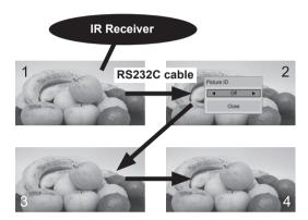
When using the 4 Set (Total Set ID: 4) Set IDs are assigned as shown in the picture.
