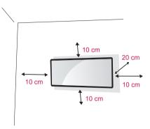
Install the monitor at least 10 cm away from the wall and leave about 10 cm of space at each side of the monitor to ensure sufficient ventilation.
