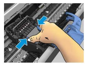
8. Lift the printhead out of the carriage.
