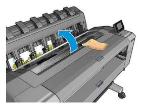
Move the carriage manually to the left side of the printer, if feasible. 2.
