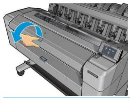
NOTE: When the roll is unloaded in this way, no barcode is printed on it, so the printer will not know the length of the roll when it is next loaded. See Printing paper info on page 57.
