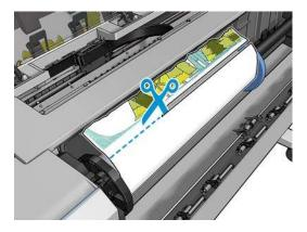
Remove the paper left in the printer.
