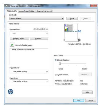
Select Layout/Output > Fit to to scale the document to a particular size. Alternatively, you can scale the document in Project.
