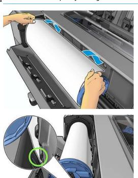
Roll the paper into the printer until you feel resistance and the paper flexes slightly. When the printer detects the paper, it feeds it in automatically.
