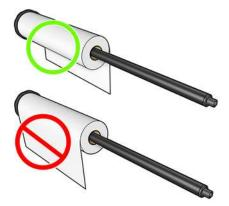
Ensure both ends of the roll are as close to the spindle stops as possible.
