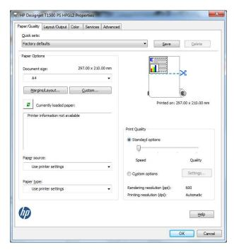
Select Layout/Output > Fit to to scale the document to a particular size. Alternatively, you can scale the document in Excel.
