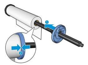
8. Ensure that the blue stop is pushed in as far as it goes; until both ends are against the stops, then close the latch.
