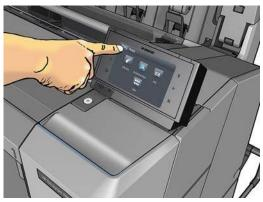
The front panel is located on the front right of the printer. It gives you complete control of your printer: from the front panel, you can print, view information about the printer, change printer settings, perform calibrations and tests, and so on. The front panel also displays alerts (warning and error messages) when necessary. Information about specific uses of the front panel can be found throughout this guide.
