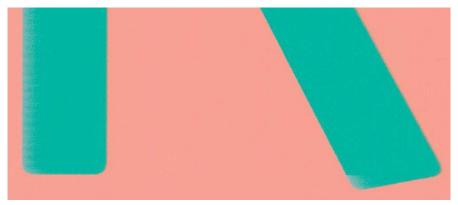
If edges of objects or lines appear to be poorly defined or lighter in density, and you have already set the print-quality slider to **Quality** in the driver dialog, select the custom print-quality options, and try setting the quality level to **Normal**. See <u>Printing on page 62</u>.
