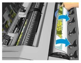
If the leading edge of the paper is ragged, trim it carefully with scissors. **7.**
