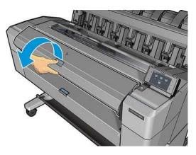
4. Load the spindle into the printer, with the blue stop on the right. Hold the spindle by its ends and not in the middle, to avoid touching the paper and perhaps leaving marks on it.
