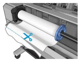
6. Insert the edge of the paper into the printer.
