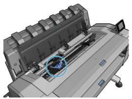
**CAUTION:** If the carriage is left in the removal position for more than three minutes without inserting or removing the printhead, it tries to move back to its normal position in the right-hand end.
