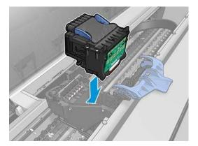
Check that the printhead is correctly aligned with its ink connectors. 2.
