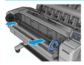
3. The spindle has a stop at each end. The blue stop can move along the spindle and has a latch to lock it in place. Open the latch and remove the blue stop from the end of the spindle.
