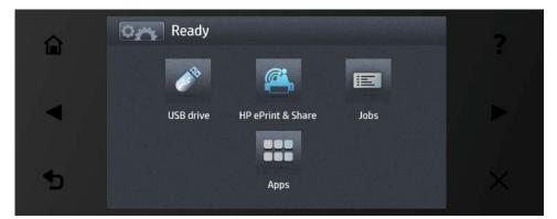
The front panel has a large central area to display dynamic information and icons. On the left and right sides you can see up to six fixed icons at different times. Normally they are not all displayed at the same time.
