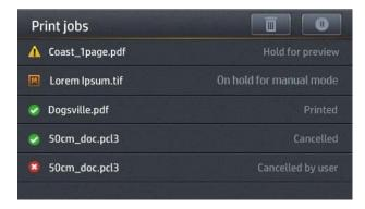
• If you put the printer into manual mode from the front panel, all jobs in the queue are put on hold for manual mode, and you can print them from the queue. When you exit manual mode, any jobs still in the queue return to their previous status.
