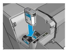
4. Push the cartridge into the slot until it snaps into position. You should hear a beep and see confirmation that the cartridge has been inserted.
