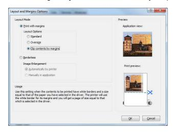
If you intend to print on roll paper, you must decide where the printer should cut the paper. In the Layout/Output tab, check or uncheck the Disable automatic cutter option, and check the Autorotate option, which can help to avoid wasting paper.
