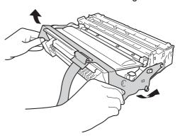
Hold the drum unit and toner cartridge assembly level with both hands and gently shake it from side to side several times to distribute the toner evenly inside the cartridge.
