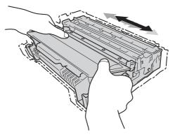
Put the drum unit and toner cartridge assembly firmly back in the machine.
