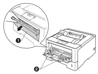
Press the front cover release button and open the front cover. Remove the silica gel pack ①.
