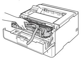
Remove the orange protective material from the drum unit and toner cartridge assembly.
