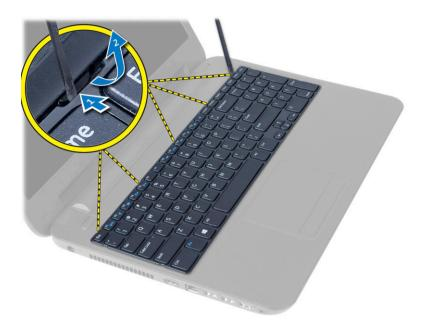
4. Slide the keyboard towards the display assembly and flip the keyboard over the palmrest.
