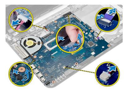
4. Remove the screw that secures the system board to the computer. Lift the system board from the computer.
