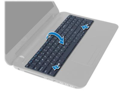
5. Disconnect the keyboard cable from the connector on the system board and lift the keyboard off the palmrest.
