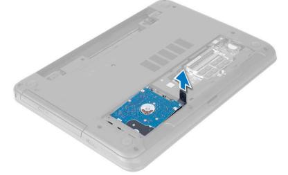
5. Remove the screws that secure the hard-drive bracket. Lift the latch to remove the hard-drive bracket from the hard drive.
