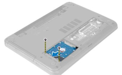
4. Slide the hard drive to release it from its connector. Lift the tab to remove the hard drive from the computer.
