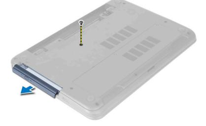
**4.** Remove the screws that secure the optical-drive bracket to the optical drive. Remove the optical-drive bracket from the optical drive.
