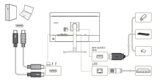
Use the product as a hub to connect the PC to a variety of devices and/or networks. To establish a LAN connection, use a Thunderbolt™ 3 / 4 cable: \_\_\_\_\_ \$, \$ port or USB Type-C cable: \_\_\_\_ \$ port.
