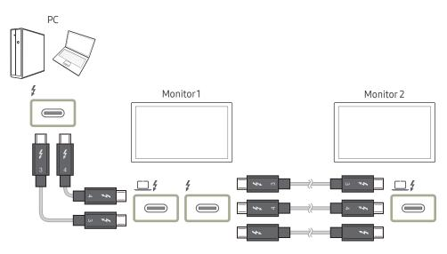
Dual display (daisy chain) support depends on your PC and the connected Thunderbolt™ 3 / 4 cable. The Thunderbolt™ 3 port on your PC must support dual 4 K @ 60 Hz output, and the particular 40Gbps Thunderbolt™ 3 / 4 cable (☐ 👟 ज ) need to be purchased separately. For detailed specification of the Thunderbolt™ 3 / 4 cable, visit the official Thunderbolt website.
